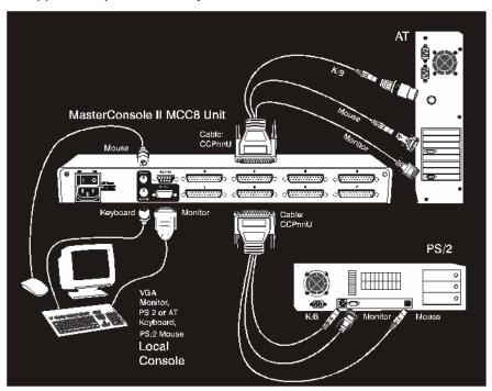
Figure 7 One-Tier Configuration Cabling Detail
